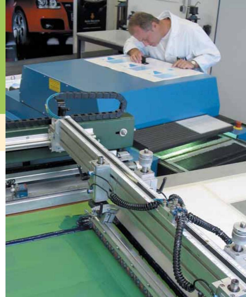
as on the following pages. Thus the screen printer should try to work with a fine fabric and low thread diameters. Screens should be coated with high quality, finely dispersing copy emulsions. Coating should be thin, however should not be too rough (Rz values; roughness values).
