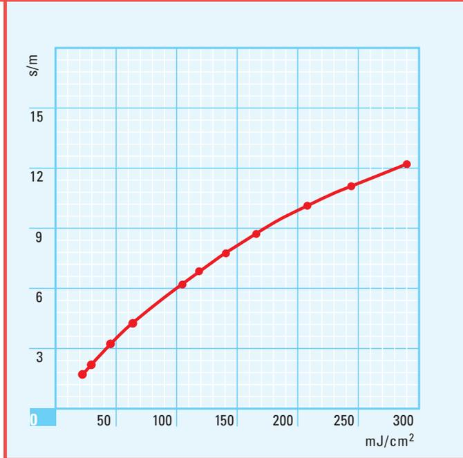
Comparison tests in our laboratory showed that the lamp output values measured with the Tesa/Hönle system are similar to those measured with the Kühnast integrator. With lower dosages the Tesa/Hönle system shows lower values than the Kühnast integrator and in a range of 200 mJ/cm² results of both systems are quite comparable.
