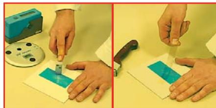
Printers will have to use the known test methods like fingernail and cross hatch adhesion tests to evaluate sufficient curing and adhesion of an ink. If the ink film has a sufficient polymerisation these tests will show sufficient hardness, good adhesion and scratch resistances. If an ink is still soft like wax curing was
