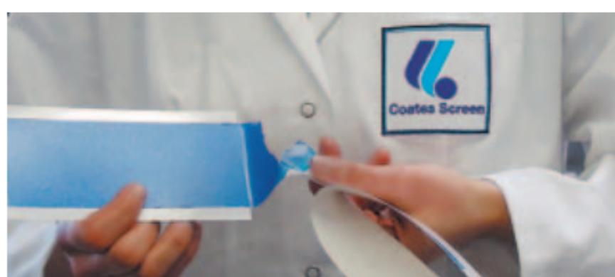
*Various ink ranges printed on different types of self-adhesive foils. Some inks show a high tendency to edge curl. In addition to the ink type tearing resistance strongly depends on the substrate.*
